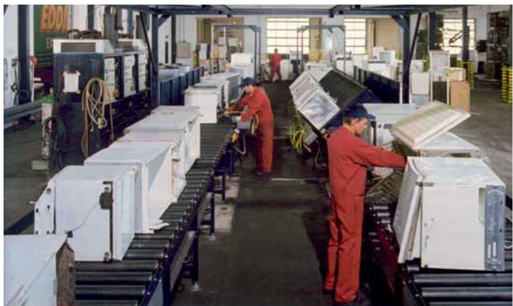
Refrigerator Disassembly Plant Neukölln: Emptying the refrigeration cycle
