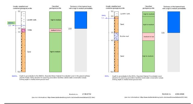
Fig. 4a: Diagram of a borehole incl. information on the thickness of the layer with a high to medium hydraulic permeability and the depth to groundwater.
