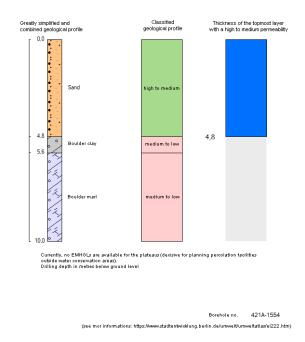
Fig. 4b: Diagram of a borehole incl. information on the thickness of the layer with a high to medium hydraulic permeability
