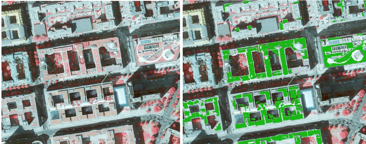
Fig. 2: Supervised classification results, left: TrueOrthophoto, 2020; right: automated preliminary mapping of the green roof inventory (green)
