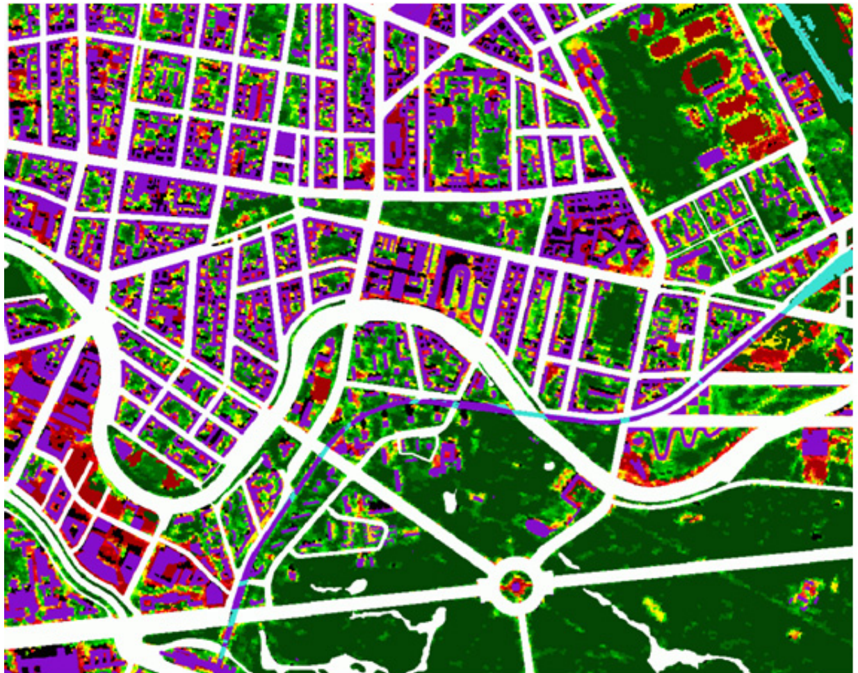
Fig. 6: Uncorrected Degree of Impervious Coverage (Grid Data) – Intermediate Results of Rule-based Classification
