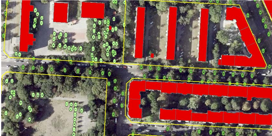
Fig. 2: Section of the geo base data and factual data used: ALKIS building layer (red), ISU5 block (segment) borders (yellow), roadside trees/ objects (dark green), trees/ objects in parks or recreational areas (light green) with the true orthophotos from 2020 in the background (Source: SenStadtWohn - Geoportal Berlin)
