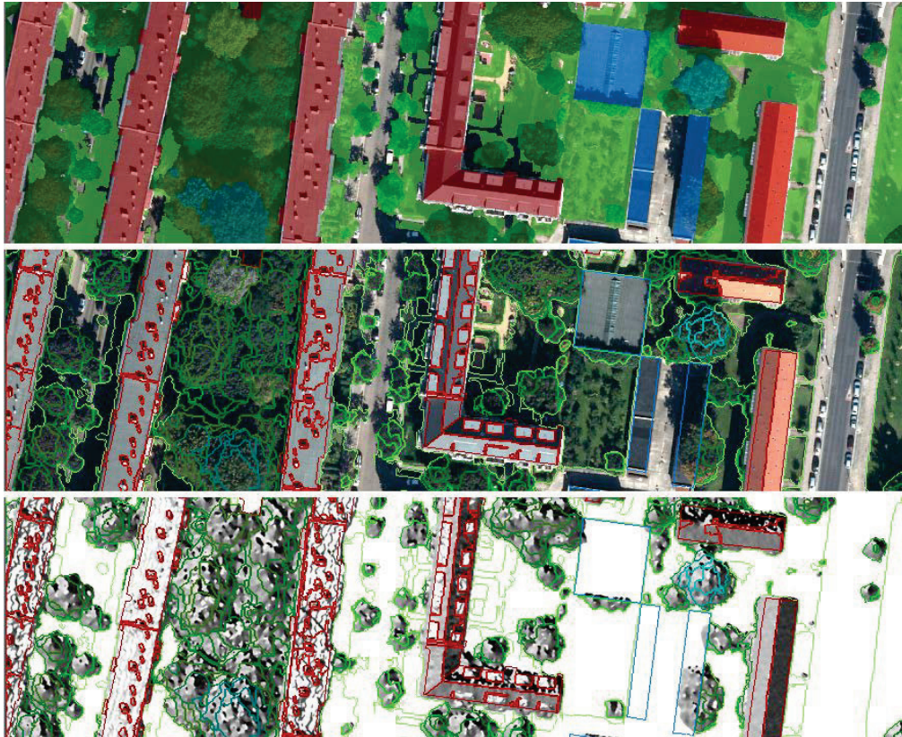
Figure 46: Result of the new MRF as the basis for further separation of roof areas
