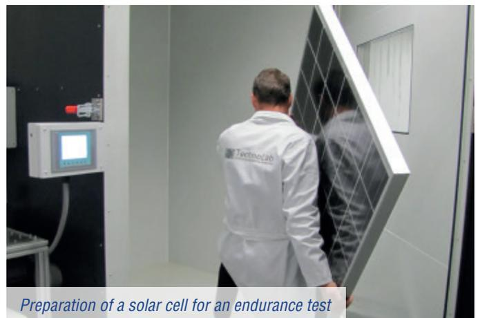
Preparation of a solar cell for an endurance test
