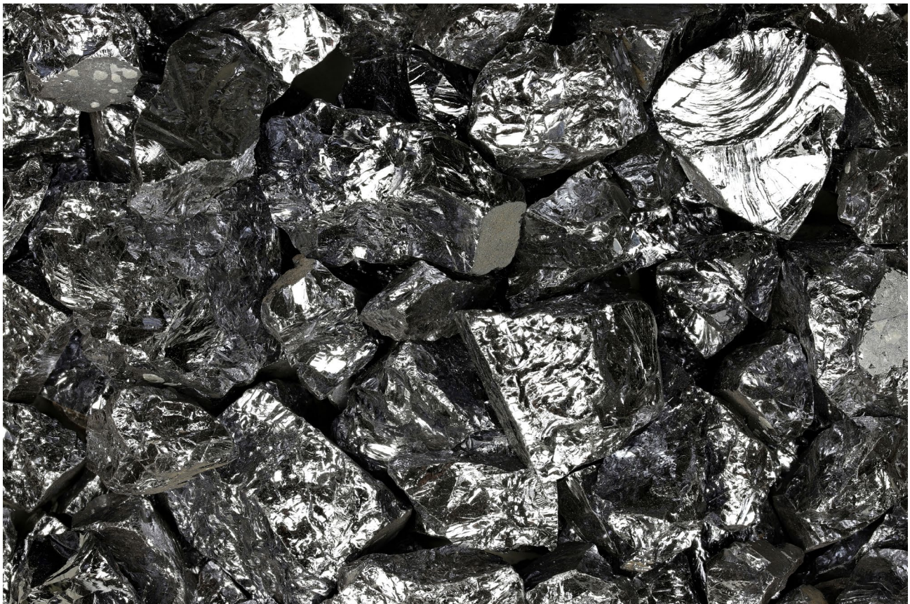
Polycrystalline silicon, as seen here, is obtained from raw silicon and is essential for the majority of all solar modules worldwide.
